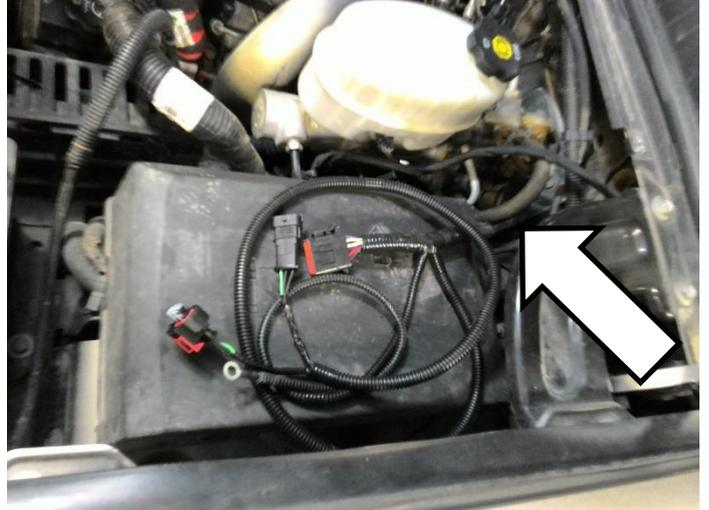
Feed the 20 pin round connector of the BD harness up over the transmission and down the back side by the main transmission connector.
