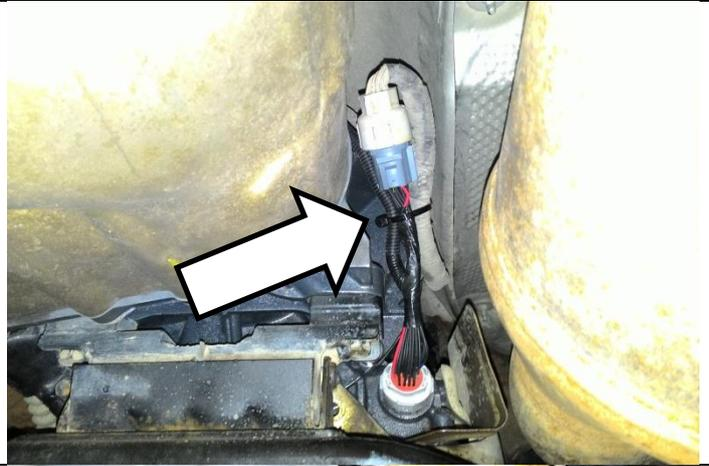
Zip tie the new harness to the existing vehicle harnesses, out of the way of the front drive shaft and other moving parts on its route to the engine bay.
