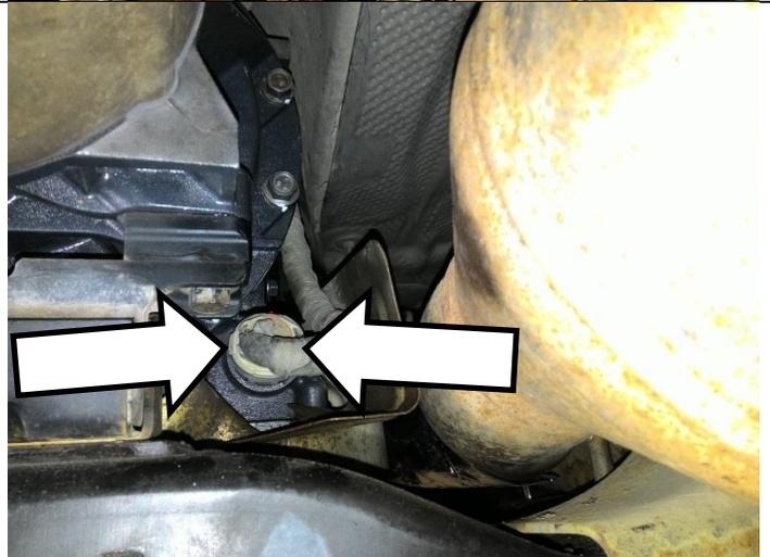
Connect the BD harness inline and carefully zip tie the harnesses so that they stay away from the exhaust pipe.
