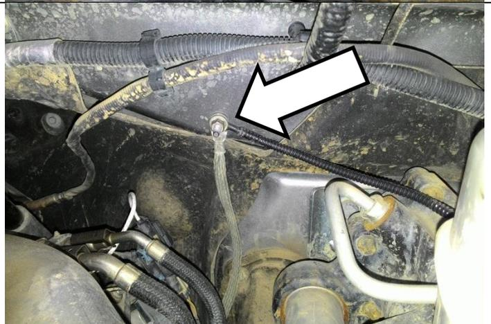
Locate the engine MAP sensor and plug the BD harness inline. Zip tie the wiring to keep it away from moving or hot parts.
