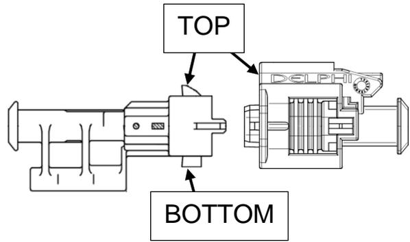
Connect the module to the gray plug from the transmission/engine wiring harness.
