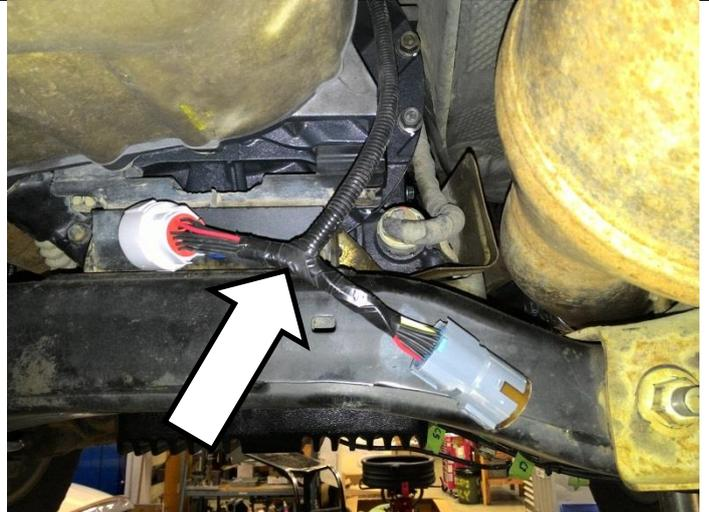
Disconnect the transmission 20 way round electrical connector by squeezing on both sides and wiggling it off. You may either use the special Allison tool for this, long needlenose pliers or remove the heat shield to get your fingers on the connector.
